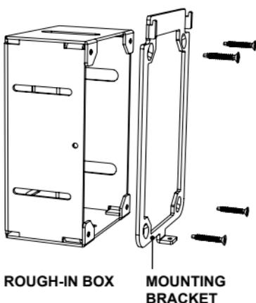
Attach the rough-in box to the structure. The rough in box can be adjusted in / out to accommodate different finish thicknesses. Use the narrow slots to attach the screws, the wider slots are used for tool access. Attach the adhesive gasket to the mounting bracket (note the alignment of the holes on the bracket and the gasket making sure they line up before adhering it). Next, attach the mounting bracket to the rough-in box using the included #6 Phillips head screws.
