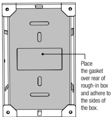
Place the vapor barrier in the rear of the rough-in box and adhere the flaps to the inside of the box. Once the vapor barrier is in place, cut a slice to allow cable routing.
