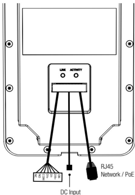
**Note:** the RJ45 connector block should be on the right side of the terminal connector, as shown here.
