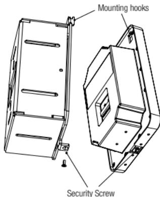
Using the included screw driver and M2 screw, attach the video doorbell to the bottom tab of the mounting bracket.
