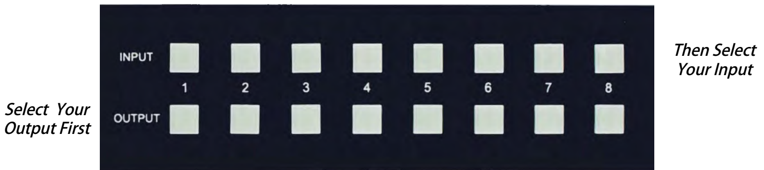
Figure 1 ~ AC-MX88-UHD Panel Controls
