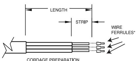
\*Furman recommends use of wire ferrules (not included) to terminate stranded wire in coupling connector.
