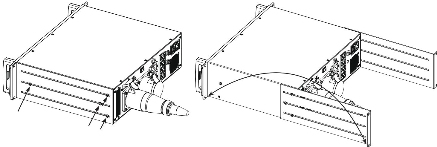
Remove the securing screws from the side and front portions of the P-6900 AR E's adjustable rear rack ear and reinforcement side plate (located on either chassis side). Reverse the rack ears and re-attach to the P-6900 AR E chassis (as shown on the right).
