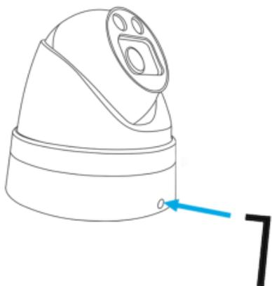
3. Rotate the mounting bracket base, aligning the screws with the exit holes and remove the base.
