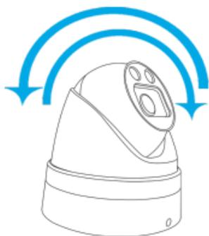
7. Snap the camera body into the base and rotate the screws into their slots until secure.
