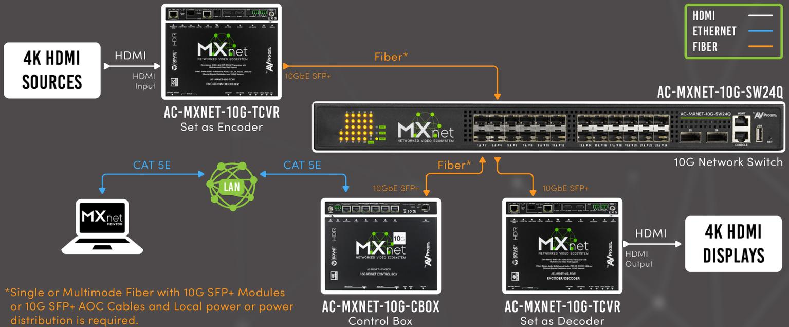
\*Single or Multimode Fiber with 10G SFP+ Modules or 10G SFP+ AOC Cables and Local power or power distribution is required.
