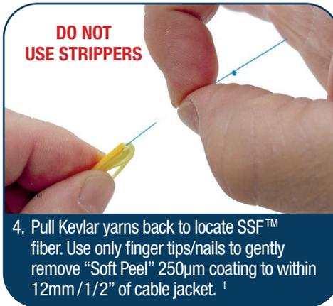
4. Pull Kevlar yarns back to locate SSF™ fiber. Use only finger tips/nails to gently remove "Soft Peel" 250µm coating to within 12mm / 1/2" of cable jacket. <sup>1</sup>
