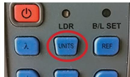
3. On the OPM, press the “UNITS” button until upper right portion of screen is blank and dBm is listed to the right of the main screen read-out (see step 1B image).
