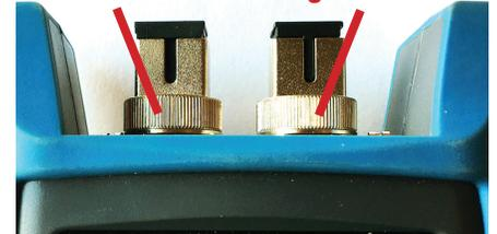
4. Plug REFERENCE cable into the appropriately labeled port on the OLS. SC testing: single-ended testing/ 1 cable. LC testing: double-ended testing/ 2 cables.
