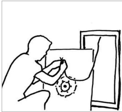
Strip the wire by 10 mm. Connect the speaker cable to the speaker, be aware of the polarity
