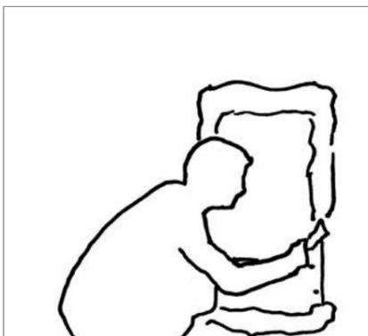
Fill in plaster, we HIGHLY recommend to use a fl exible filler, e.g. Knauf Unifl ott or Ardex 828
