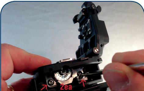
4. Loosen the two guide screws with the supplied wrench. Only approx. one turn is required, do not loosen completely.
