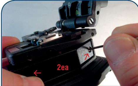
2. Using the Allen wrench remove the two screws that secure the guide cover. **\*Not all models**
