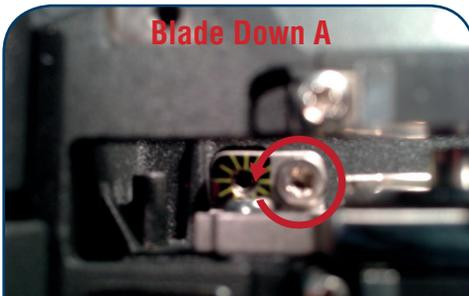
A. Loosen the hex screw located behind the blade looking down on the unit, counter clockwise one full turn. **\*Located in front on some models.**
