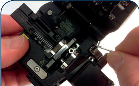
1. Using the Allen wrench included with the cleaver, on the top right side remove the screw that secures the fiber scrap box. Set the scrap box aside. **\*Varies by model**
