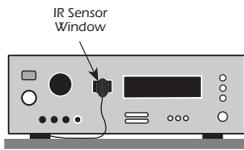
Fig. 5a IRE-1.0 attached directly to IR sensor window
