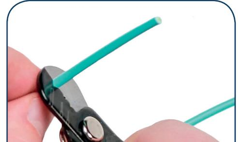
5. Using the appropriately sized opening on strippers for cable being spliced, remove approximately 50 mm/2" of the cable jacket. If needed, install build-up tube.
