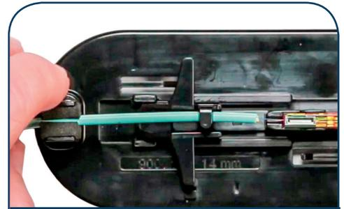
11. Insert cable under slide arm and place into foam holders so cable lays straight. Repeat the previous cleaving process for the right cable fiber leg to be joined.
