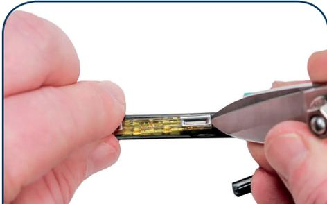
3. Remove the yellow fiber splice with fingers or sharp edge. Avoid touching fiber opening. Place in splice installation tool.
