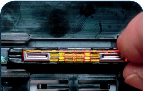
12. Insert the right fiber forward into splice, watching for movement of the left fiber as it is pushed from within the splice and/or loss of light if using a VFL.
