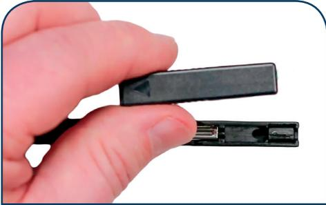
1. Remove the left and right covers from mechanical splice, placing one on each leg of cable to be joined with arrows pointed towards the needed splice.
