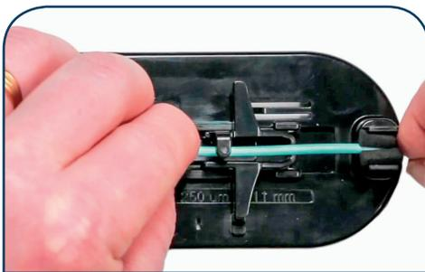
13. Upon movement, loss of light, or both, maintain forward pressure with a bow in the cable and place cable under slide arm and into foam cable holder
