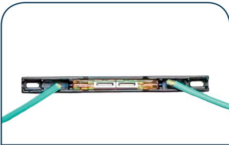
15. Carefully remove splice and fiber cable from tool and place into splice assembly.
