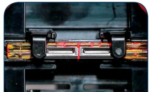
14. Maintain forward pressure and loss of light while pushing each of the two slide arms towards the center. Slide the metal tabs until they touch to lock in the fibers.
