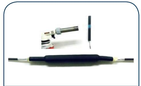
18B. OPTIONAL: Using torch, apply heat from center to the ends. Verify no air is captured inside.
