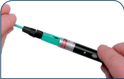
9. If possible, connect VFL on the opposite end of one of the fibers being spliced for verification purposes.
